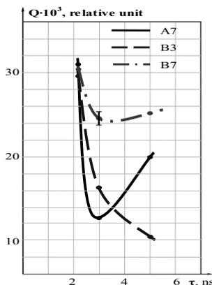
Fig. 4. Experimental dependence of Q factor of noise oscillator on length of pulses.
