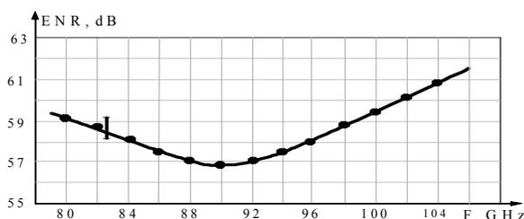
Fig. 1. Characteristics of noise factor in operating range.
