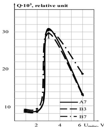
Fig. 3. Experimental dependence of Q factor of noise oscillator on amplitude of pulses.
