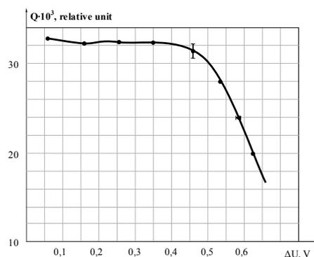
Fig. 2. Experimental dependence of Q factor of noise oscillator on back bias voltage.
