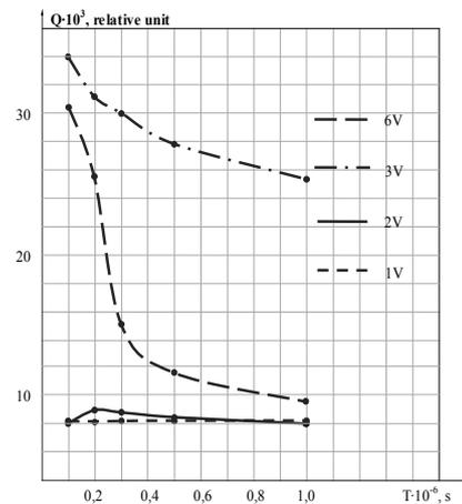
Fig. 5. Experimental dependence of Q factor of noise oscillator on time of repetition of pulses.
